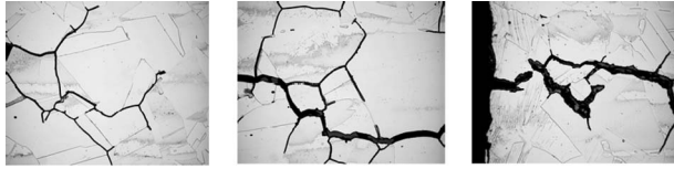
Fig. 1 The picture after crack coalescence, provided by Professor Chen Zemao (Vice Dean, School of Aerospace, Xi'an Jiaotong University)
